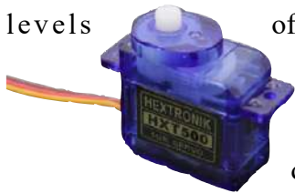
Fig. 20.1: HXT500 Aileron Servo (Ref. 45)
