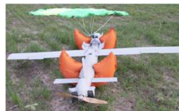
Fig. 7.2: Airbag Recovery System (Ref. 29)
