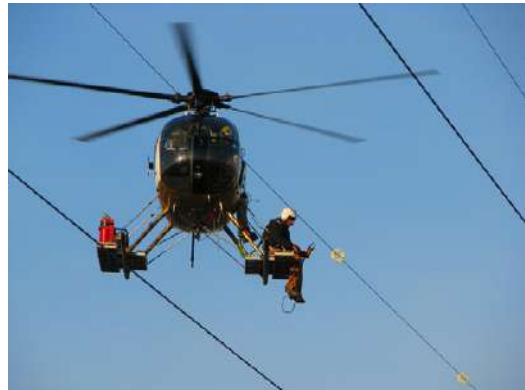
Fig. 2.1: Helicopter Power Line Inspection (Ref. 8)
