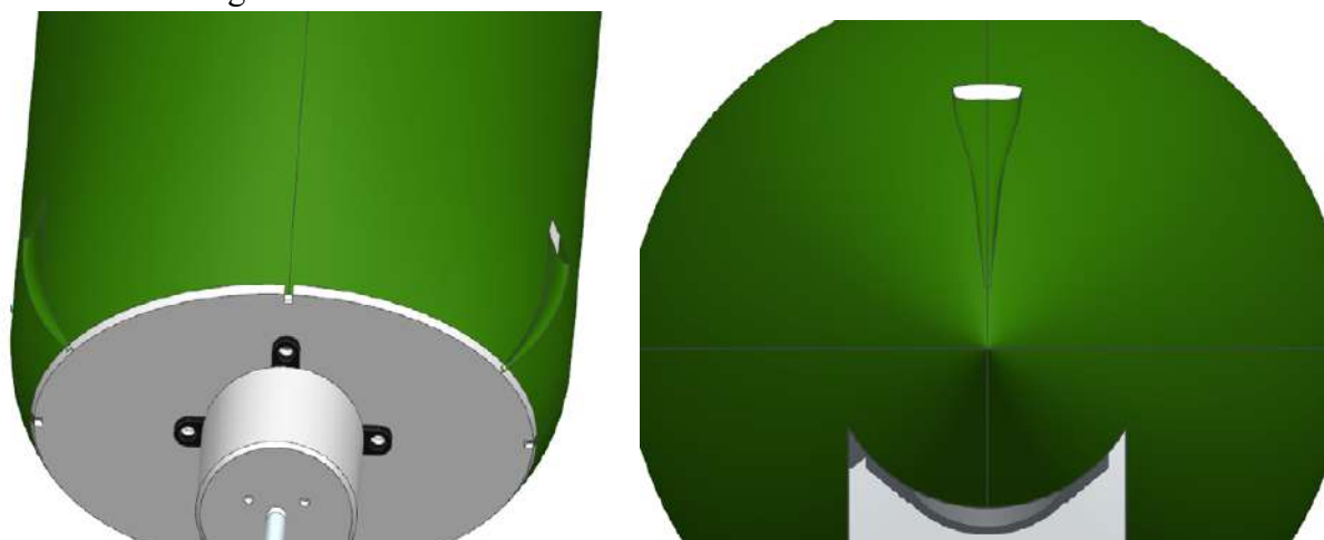
Fig. 20.9: Fuselage and Sensor Pod NACA Inlets (NTS)
