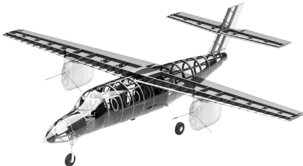
**Figure 8.1: Structural layout of HT-LIT aircraft.**
