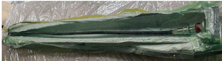
Figure 50: Fuselage Layup under Vacuum
