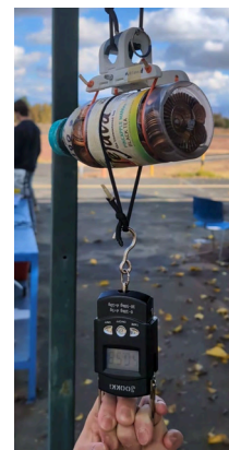
Figure 63: Early Stage Pylon Structural Testing
