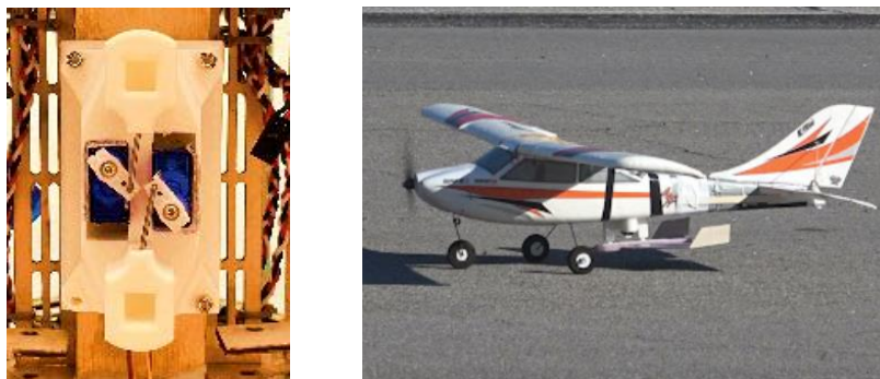
Figure 7-3: Common mounting system (left) and X-1 prototype mounted to COTS airframe (right).
