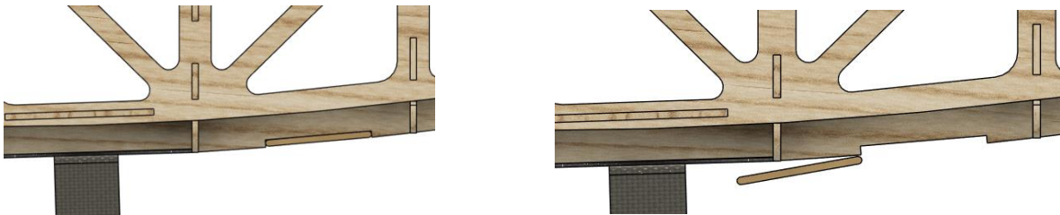
Figure 5.16. Bomb Bay Hatch (Closed vs Open)
