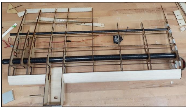
Figure 6.2. Wing Ribs and Spars Attachment
