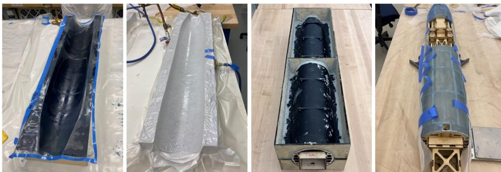
Figure 6-1: From left to right: fiberglass skin layup in 3D printed mold, vacuum bagging and cure, skin-substructure clamp using the same molds, and final product with good adhesion.
