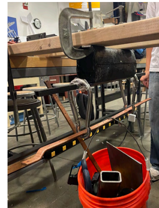
Figure 57: Fuselage Structural Test Setup
