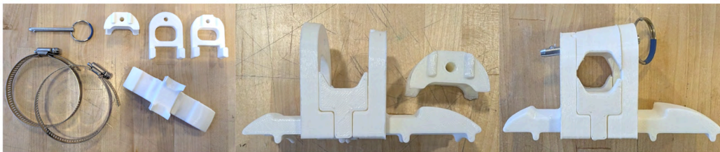
Figure 40: Pylon Components Before Assembly (Left), Assembled Pylon Pieces (Middle), and Full Pylon (Right)
