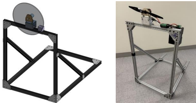
Figure 7-1: CAD (left) and practical assembly of static thrust stand (right).
