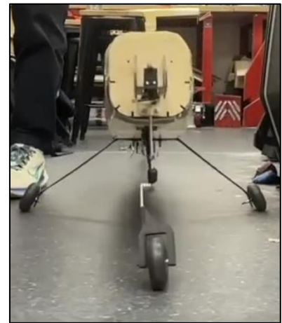
Figure 7.6. Fuselage Drop Test Loaded to MTOW weight
