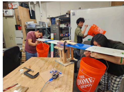
Figure 59: Wing Structural Test Setup
