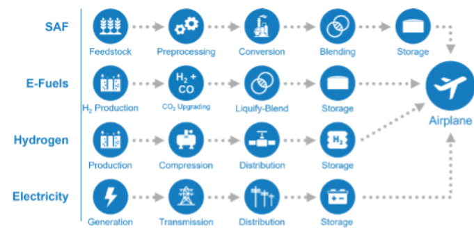
Fig. 6 Conceptual representation of next-generation aviation energy supply chain.
