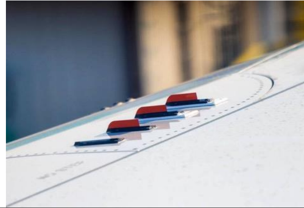
Shape Memory Alloys as Smart Vortex Generators
