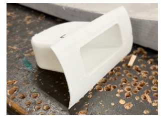
Figure 59. 3D printed cargo housing.
