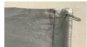
Figure 61. Tissue Lamé banner with the airfoil leading edge rod and split ring attached.
