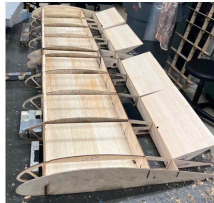
Figure 56. Wing spar-rib structure.
