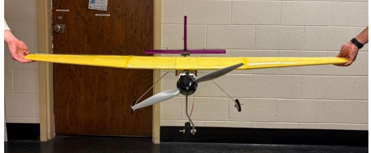
Figure 8.3 Wingtip Load Testing of Buzzerang 0
