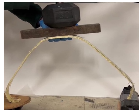
Figure 71. Gear loaded with 42 lbf.
