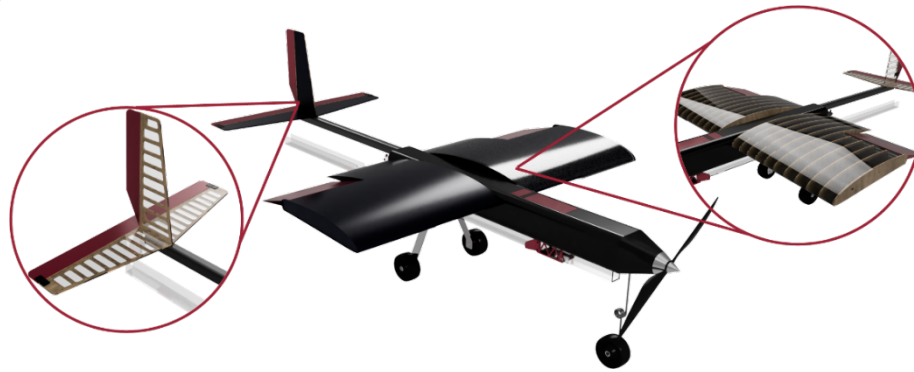
Figure 7: Full Plane CAD with wing lightening holes and tail ribs/spars shown.
