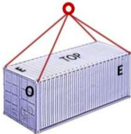
Figure 1. Sensor Shipping Container Rigging.
